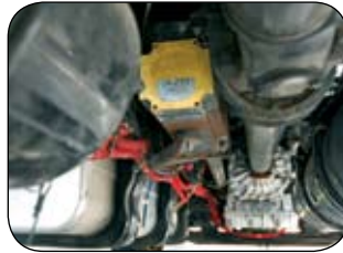
Permanent Magnet Generator driven via PTO
