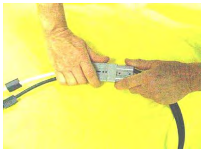
High-Voltage Input: Yazaki Connector
