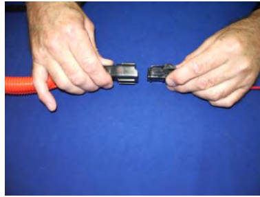
High-Voltage Input: Yazaki Connector
